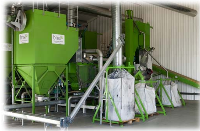
Fluidised bed combustion technology for heat and electricity by Irish company bhsi - bioenergy from poultry manure for poultry farms. Photo courtesy of bhsi
