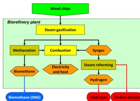
**Fig. 5: 4-platform (electricity&heat, hydrogen, biomethane, syngas) biorefinery using wood chips for biomethane (SNG), hydrogen and carbon dioxide“**
