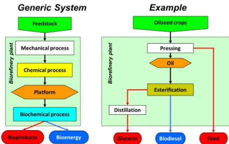
**Fig. 2: The generic system and an example for a biorefinery using the 4 features**
