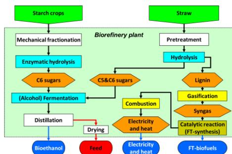
**Fig. 6: “5-platform (C6 sugars, C5&C6 sugars, lignin, syngas, electricity&heat) biorefinery using starch crops and straw for bioethanol, FT-biofuels, feed, electricity and heat”**
