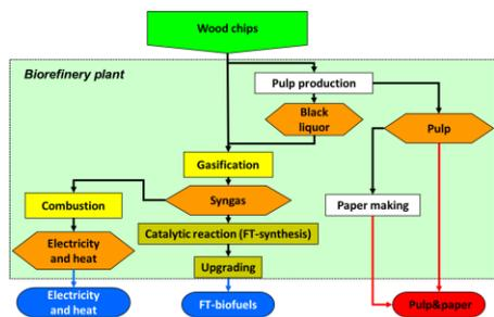
Fig. 9: “4-platform (pulp, syngas, electricity&heat) biorefinery using wood chips for FT-biofuels, electricity, heat and pulp”
