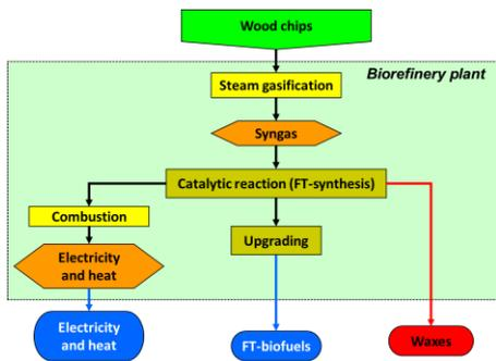
Fig. 8: “2-platform (electricity&heat, syngas) biorefinery using wood chips for FT-biofuels, electricity, heat and waxes with steam gasification”
