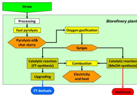
**Fig. 7: “3-platform (pyrolysis oil, syngas, electricity&heat) biorefinery using straw for FT-biofuels and methanol with oxygen gasification”**
